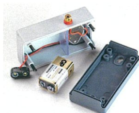
Alarm tone generator, dismantled
